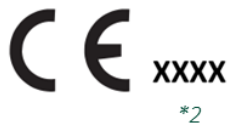
*2 XXXX = Identification number of notified body responsible for the EU-type examination and supervising ongoing conformity
